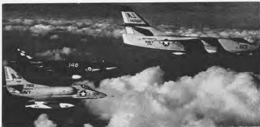
A FORRESTAL-BASED A-3B Skywarrior (A3D-2) trails an in-flight refueling boom as a Royal Navy Scimitar nuzzles up to the nozzle. An A-4 Skyhawk (A4D) of VA-83 watches the hook-up.
