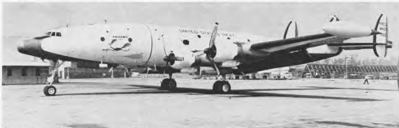
PAISANO DOS is the name given this EC-121K Warning Star (WV-2) assigned to NAS Patuxent and operated as an airborne geophysical laboratory during Project Magnet. Data gathered will be used to improve international navigation and learn more of inner and outer space.
