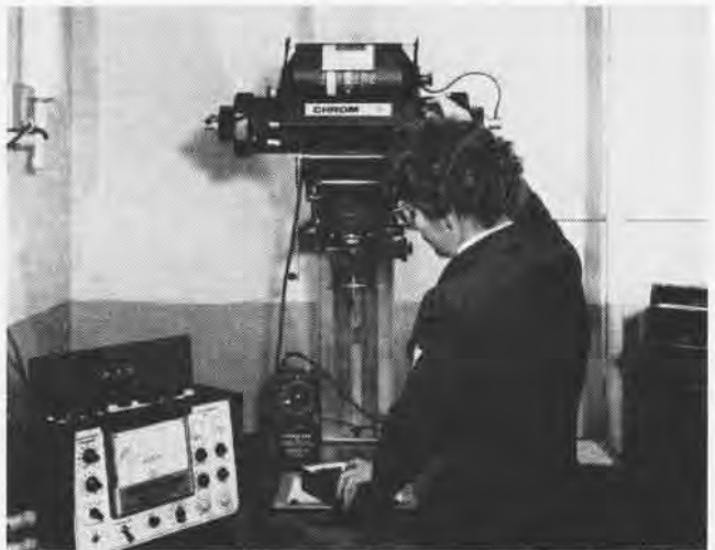
S. K. SPENCER, PH1 , uses the color densitometer probe to take a reading on a color negative while working in NPC's color printing dark room.
